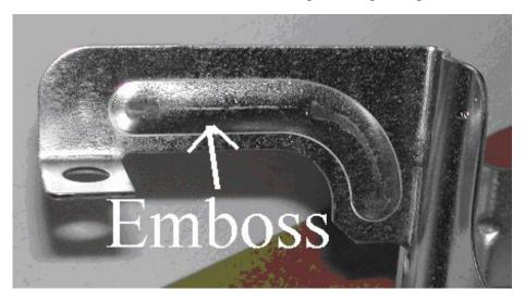
Source 1 inventory has been purged and brackets are now being used in production. New bracket will be assigned part number S1-37319831002.
